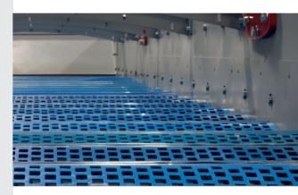
Smart innovation: The SPALECK MultiZONE deck -Several screening-areas available on one screendeck. In this way the screening-quality can be easily controlled and the screening-machine can be flexibly adapted to a wide range of materials.
