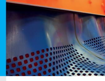
SPALECK FineSideCOVER The leading side-wall sealing with unique change options: Depending on the application, the customer can choose between a flat and a trough-shaped screen-surface.
